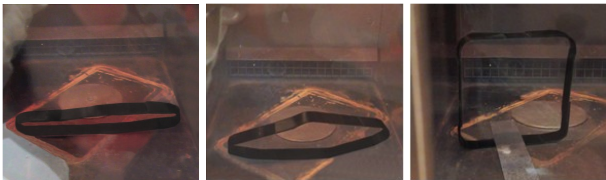
Figure 8. Frames from a video recording of the shape recovery process
