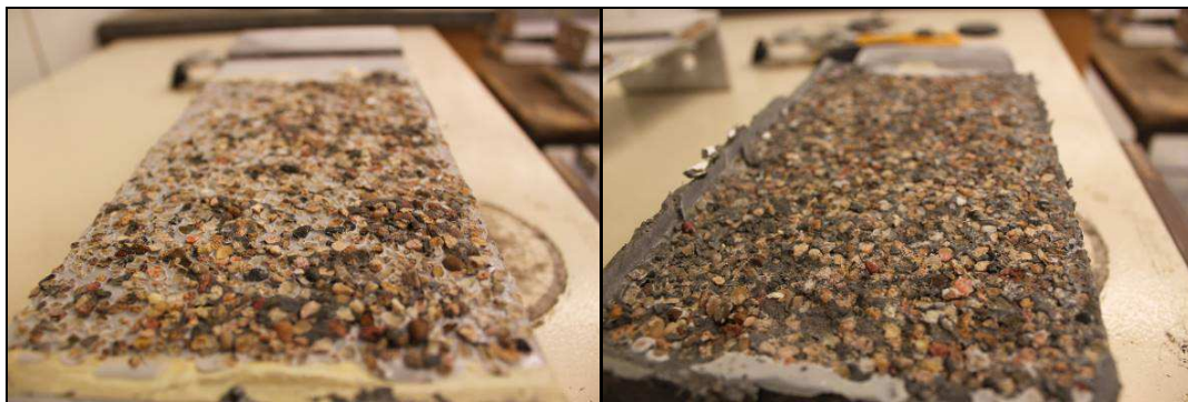
Figure 3. Failure mode of control specimen showing the debonded surfaces on the GFRP pultruded plate (left) and on the UHPC (right).
