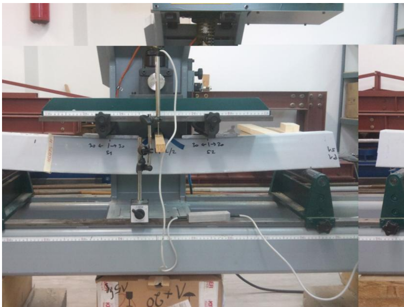
Figure 4. The testing of the GFRP carrier – four-point-bending-test – 4PBT.
