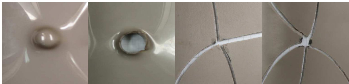
Figure 4. Failure of PEEK material: ductile (for individual thin plates) and brittle (for internal core of sandwich material and Ti6Al7Nb skin). Different impact velocity from left to right: 1 m/s, 5 m/s, 5 m/s, 15 m/s.
