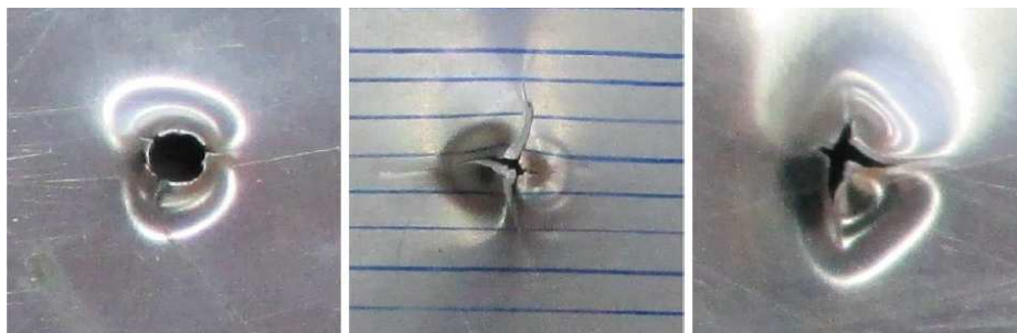
Figure 4. Progressive damage from shear to petalling for each laminate of 2024Al-Ti6Al4V-2024 Al multilayered metal sandwich (impact velocity=305,8 m/s corresponding to arrest of projectile).
