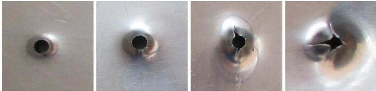
Figure 3. Progressive damage from shear to petalling for each laminate of multilayered metal sandwich of 2024 aluminum (impact velocity=435 m/s).
