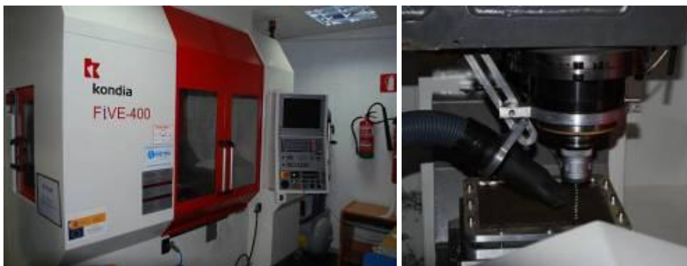
Figure 3. (a) HSMC Kondia used in the dry drilling tests. (b) CFRP drilling procedure
