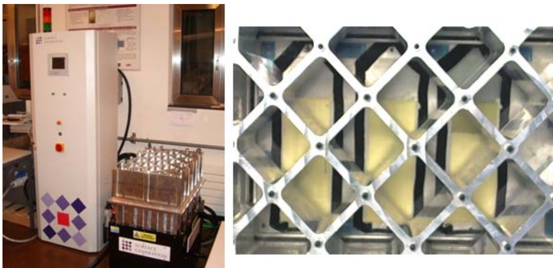
Figure 1. Heated injection test rig used to produce RTM laminates used in this paper.
