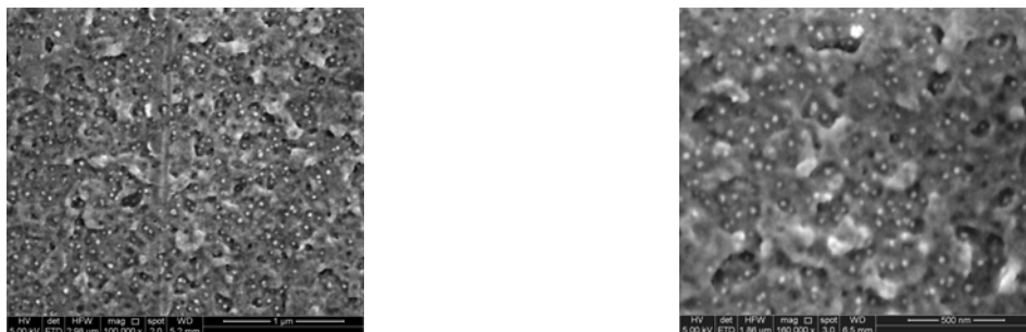
Figure 2. Analysis of the fracture surfaces of 5%wt nanomodified resins by using Field Emission Gun Scanning Electron Microscope.
