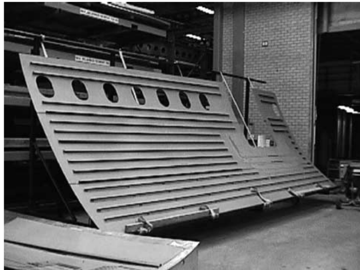
Figure 3: A skin panel including cut-outs and reinforcements (doublers and bonded stringers)
