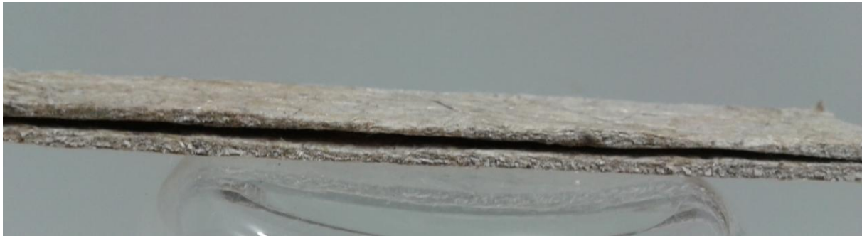
Figure 2. Thickness of 10%BC composite (top) and 10% BC Layered (bottom)
