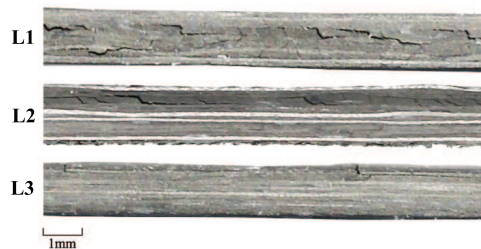
Figure 2. Damage occurred at the free-edge (Applied strain of 1.46%)
