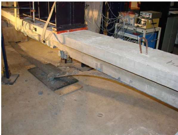
Figure 4 Beam T2 at failure
