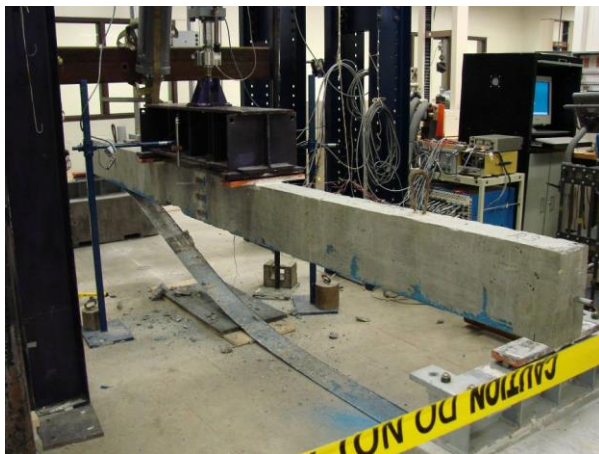
Figure 10 Beam R2 at failure
