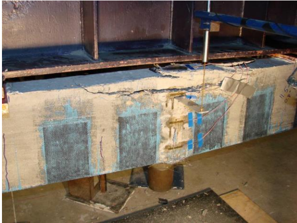
Figure 12 Beam R3 at failure
