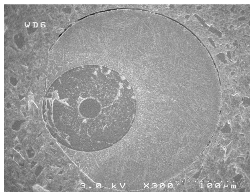
Figure 1. SEM observation of coated SCS-6 filament
