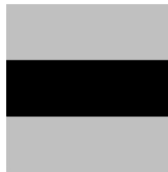
Figure 2. Geometry of the RVE for a laminated with orientation of the fibers to the \theta = 0^\circ .
