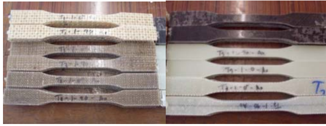
Figure 2 Dimensions of composite specimens used for tensile testing
