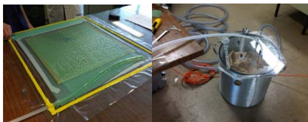
Figure 1 Production of samples using vacuum infusion impregnation process
