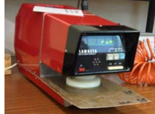
Figure 3 Alambeta Instrument for measuring thermal properties
