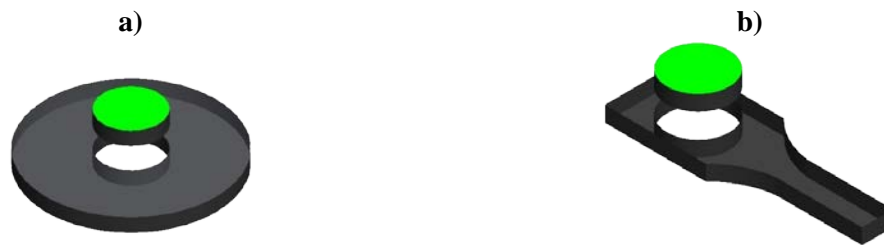
Figure 2. Schematic design of the machining operation needed to remove small disc samples (of 8 mm diameter) from (a) compression molded discs and (b) injection molded bars.
