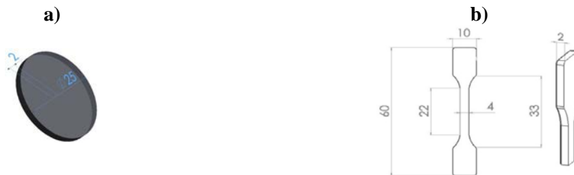
Figure 1. Dimensions (in millimeters) of (a) compression molded discs and (b) injection molded tensile specimens.
