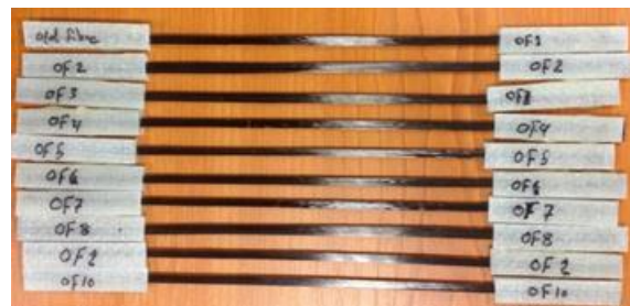
Figure 3. CFRP pre-preg tow cured specimens
