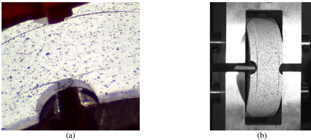
Figure 7. Initiation of the crack (a), and CFRP ring after shear delamination (b).
