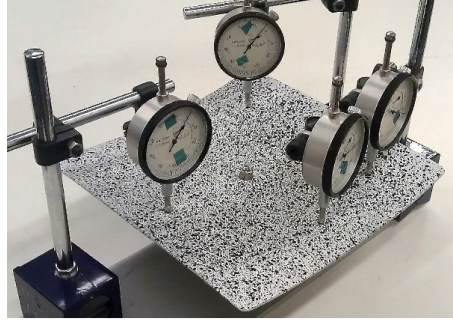
Figure 3. Test article mounted on dial gauge rig. Note that the speckle pattern visible is not relevant to this particular experiment.
