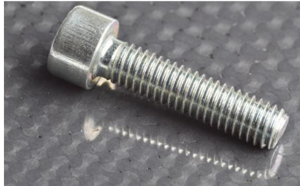
Figure 1. Reflections of a screw on a polished SiOC composite surface with reinforcement structure
