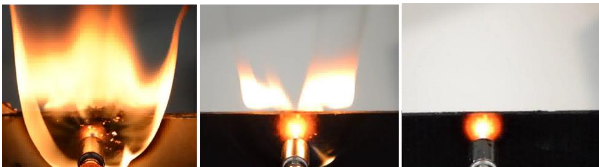
Figure 2. Comparison of E-glass SMC (left), HT-Carbon epoxy (middle) and Basalt-SiOC (right) in burner test
