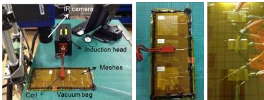
Figure 4. Left: Set-up of the induction trials. Center: Large meshes. Right: Small meshes.
