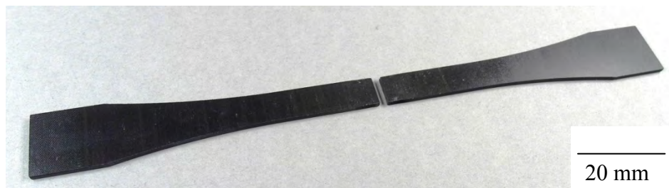
Figure 5. Fracture of specimen in the area of HAZ
