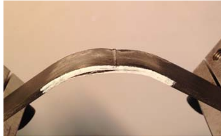
Figure 6. Compressive fracture on a specimen with an inner radius of 20 mm.
