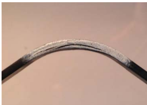
Figure 5. Delamination in a specimen with an inner radius of 15 mm.
