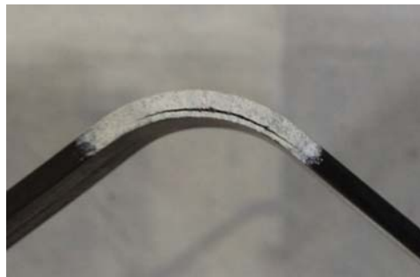
Figure 4. Delamination in a specimen with an inner radius of 10 mm.
