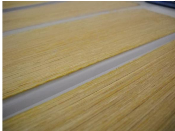
Figure 3. Unidirectional bamboo fibre preforms ready be used for composite production.
