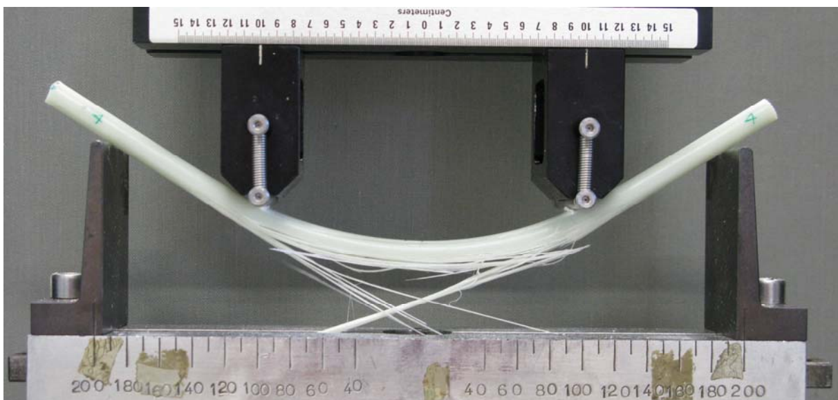
Figure 6. Failure mode of pultruded rods under 4-PB one-half span (support span-to-diameter ratio = 25).
