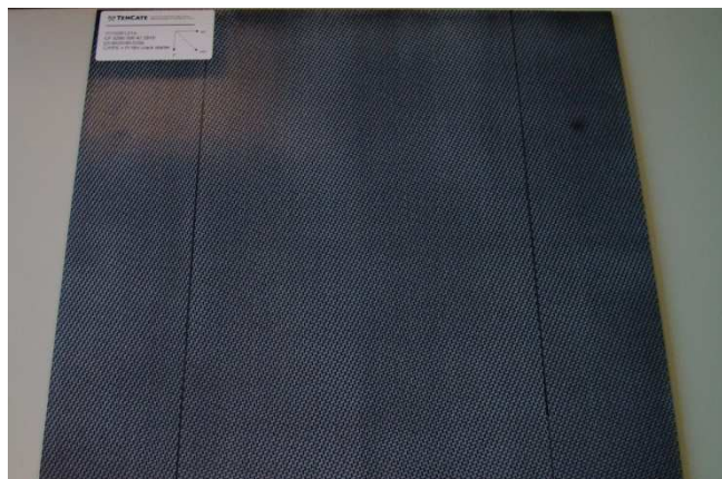
Figure 1. A 12-ply plate of CF/PPS with 13 \mu\text{m} film inserted from the two sides of the plate.
