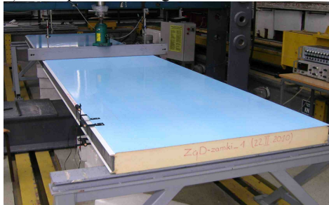
Figure 1. Set up for various shear test 1) four-point bending test, 2) three-point bending test, 3) double-lap shear test without constraint, 4) double-lap shear test with constraint, 5) torsion test
