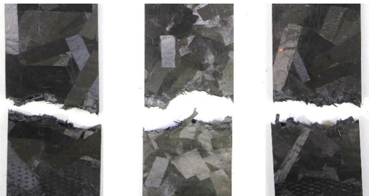
Figure 8. Fracture of UT-CTT in tensile tests.
