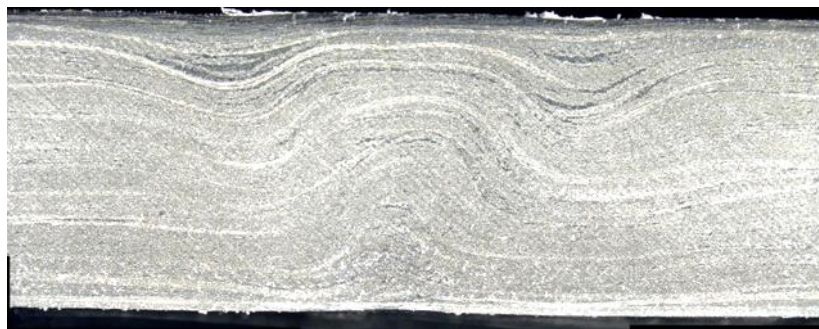
Figure 7. Cross section of specimen by the tape length of 24 mm.
