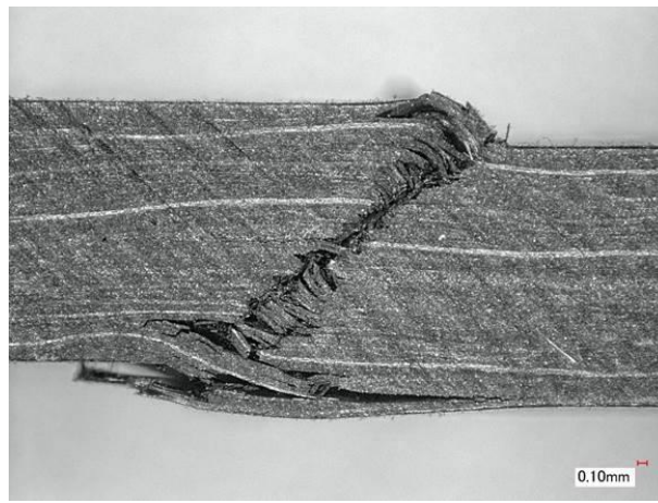
Figure 10. Buckling in the compressive tests.
