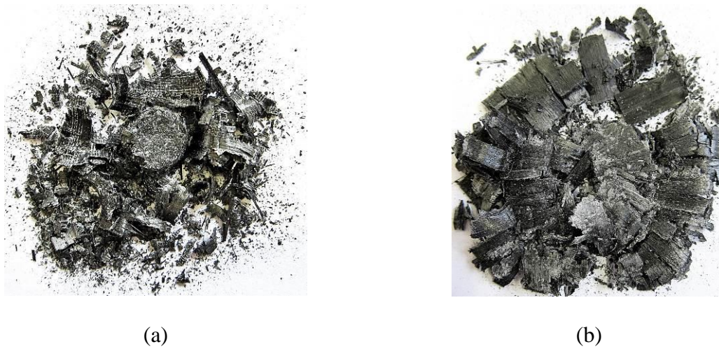
Figure 4. Remnants of the composite tubes following quasi-static testing at 1mm/minute for tubes of (a) D_o = 10.2 mm ( D/t = 6.3 ) and (b) D_o = 40.9 mm ( D/t = 22.4 )
