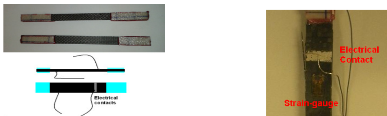
Fig. 12 Samples for tensile test of reference composite and multiscale composite
