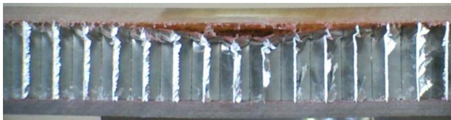
Figure 6. A cross section of a 16/16 CP E-glass/epoxy skinned sandwich panel impacted at 18J
