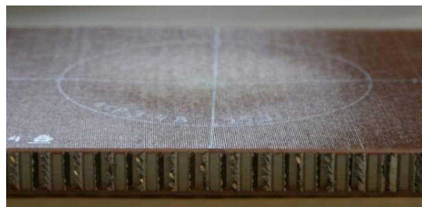
Figure 5. Dent depth in an 8/8 CP E-glass/epoxy skinned sandwich panel impacted at 25J
