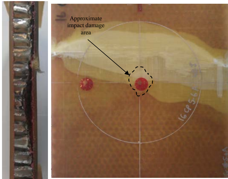
Figure 10. A side and front view of an impacted E-glass/epoxy skinned sandwich panel after CAI test
