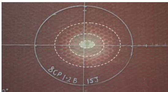
Figure 4. Damage mechanisms in an 8/8 CP E/glass skinned sandwich panel impacted at 15J
