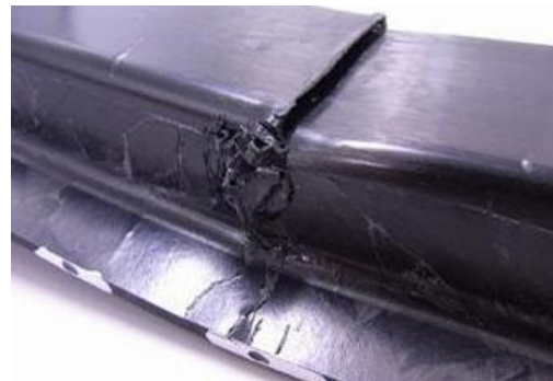
Figure.11. Hollow beam after the 3-point-bending test.
