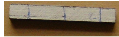
Figure 5. Failed SBS carbon/epoxy specimen
