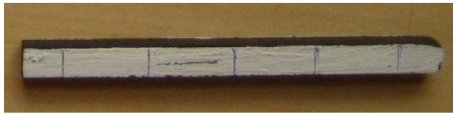
Figure 4. Failed DBS carbon/epoxy specimen
