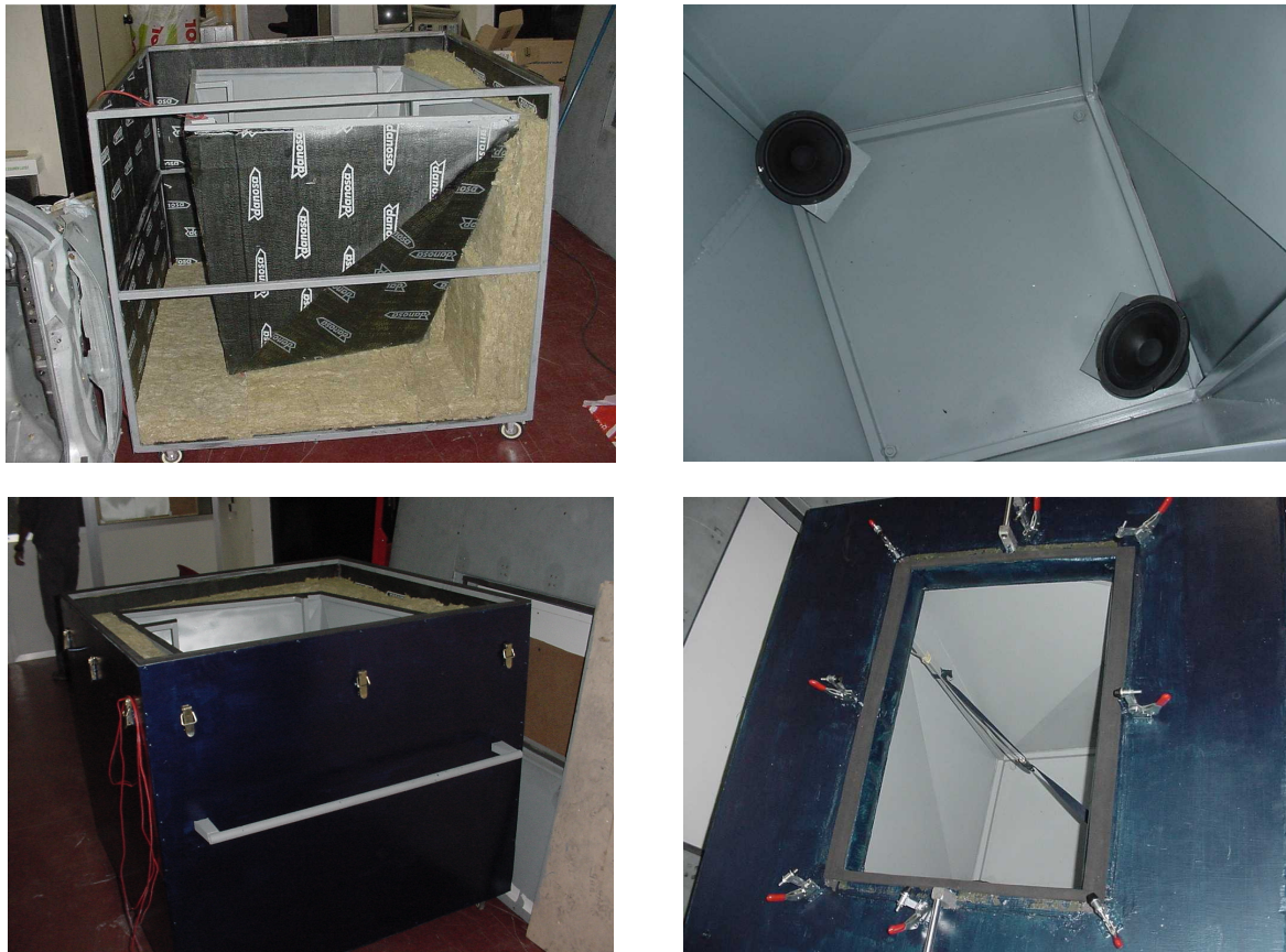
Figure 5. Small reverberant chamber used for composite panel transmission loss characterisation.
