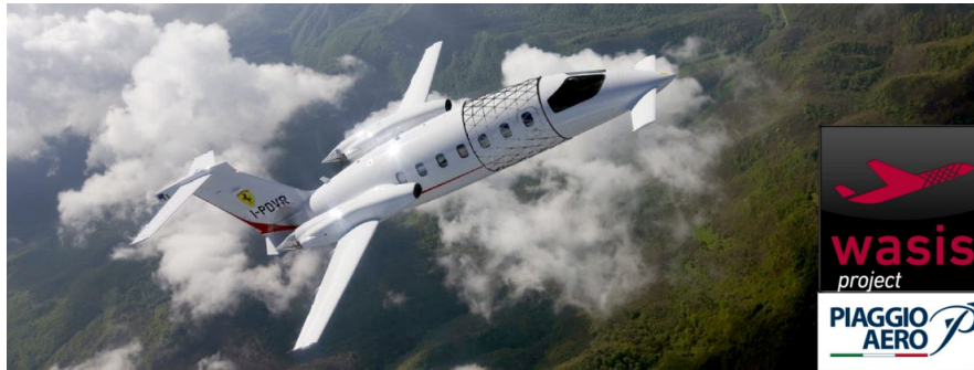
Figure 1. Piaggio Aero P-180. Avanti aircraft with WASIS lattice fuselage section superposed
