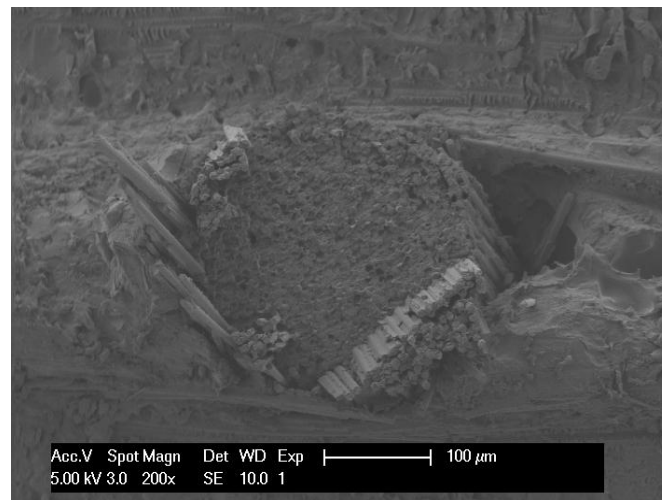
Figure 5.4. SEM image of z-pin shear failure in a SBBB specimen
