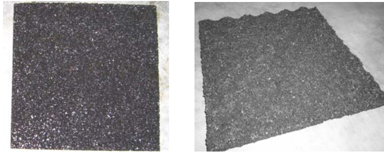
Figure 2. Wavy and flat geometries with contact surface (300x300) mm 2
