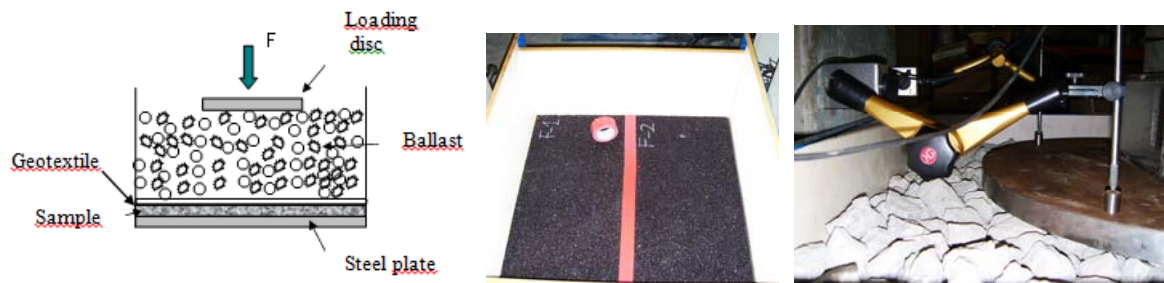
Figure 4. Fatigue test device
