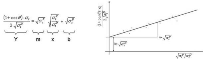
**Figure 1.** Disperse and polar fractions of SFE of a solid according to the OWRK method.
