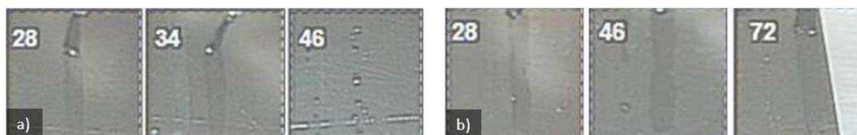
**Figure 3.** SFE of 8552/AS4-ETFE composites by means of TI before (a) and 21 days after APP treatment (b). Note that before APP, only the test fluids of 28 and 34 mJ/m<sup>2</sup> remained as homogenous films. The effects of APP after 21 days were demonstrated since any of the increasing TI pulled back into droplets.
