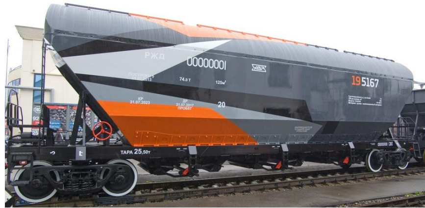
Figure 1. The manufactured hopper car 19-5167 with fiberglass body and roof
