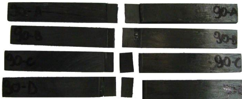
Figure 6. Photographs of the fractured 90° specimens under compression.
