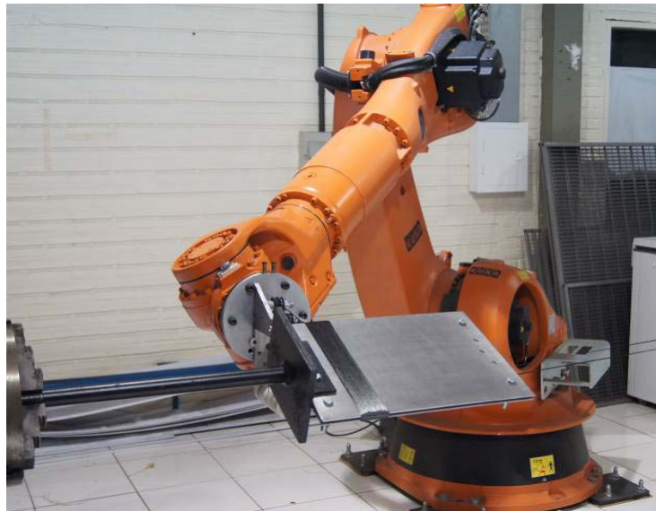
Figure 1. Manufacturing of a flat laminate by filament winding process.
