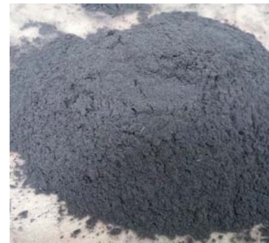
Figure 3. Collected powder after cutting carbon fiber components.
