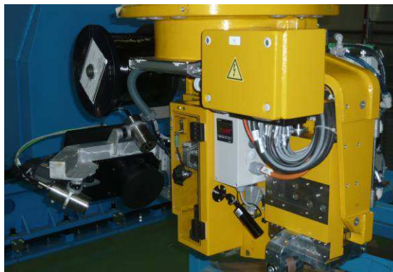
Figure 3. Head of laser assisted Thermoplastic tape placement machine in FIDAMC
