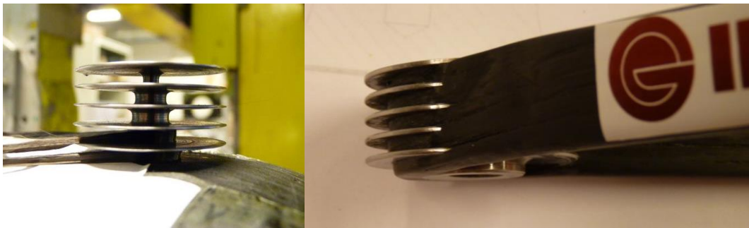
Figure 2 – Views of reels at the ribs turn-around zones.
