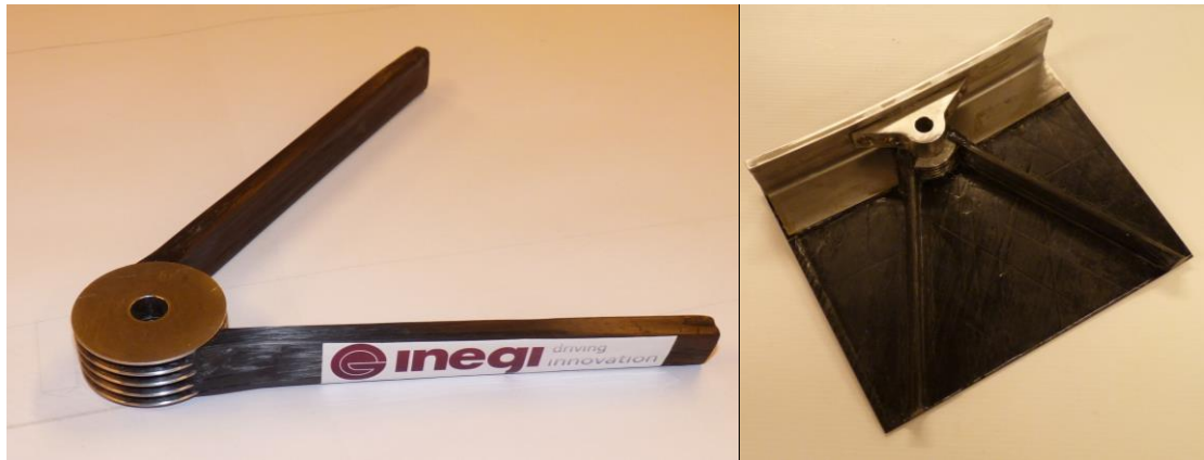
Figure 5 – Attachment frame connector details without skin (left) and with skin (right).
