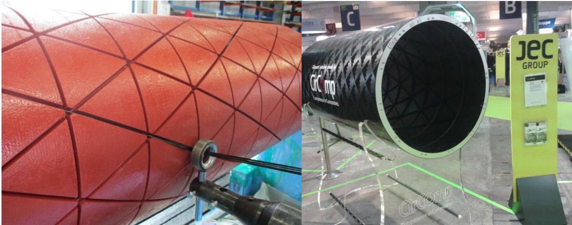
Figure 8 – 1m barrel lost mandrel (left) and final prototype (right).
