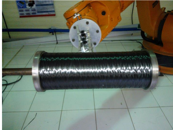
Figure 1. Manufacturing of a composite pipe by dry filament winding process.
