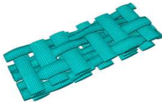
Figure 1. Meshed unit cell of G1151® interlock
