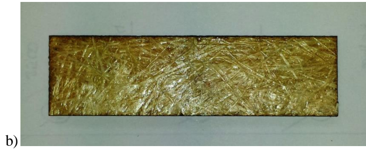
Figure 2. Specimens for flexure test: a) commercial sheet; b) sisal reinforced castor oil polyurethane composites
