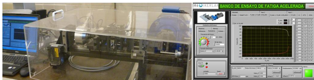
Figure 1. Accelerated flexural fatigue test rig.
