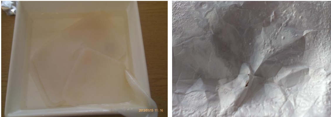
Fig.1. Images showing swollen BC (left) and BC/PHBHV composites after liophyllization (right)
