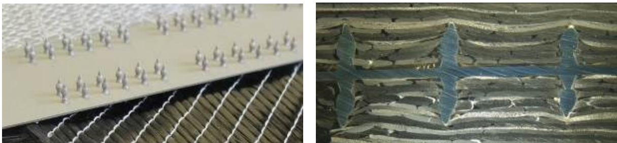
Figure 3: Thin stainless steel insert with arrays of CMT pins (left), cross-section of aligned CMT pins in CFRP laminates (right) [17]
