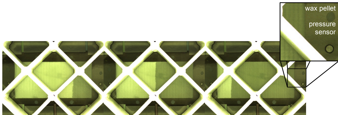
Figure 2. Flow front advancement in a 1D experiment, placement of wax pellets and pressure sensors
