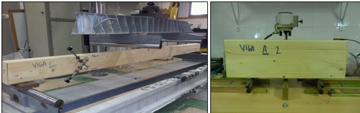
Figure 1. Left: Four-point bending tests. Right: Experimental setups for dynamic measures on small samples.
