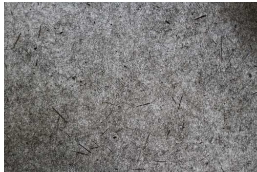
Figure 9: Undispersed fibre bundles in the RA20 mat
